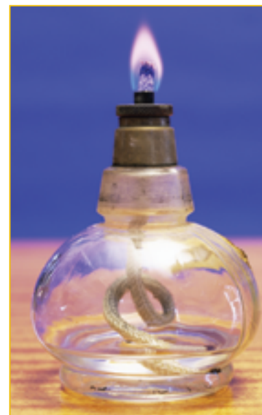
Figure 12.17 An ethanol burner. Some camp stoves such as Trangias also use ethanol (methylated spirits) as their fuel.
