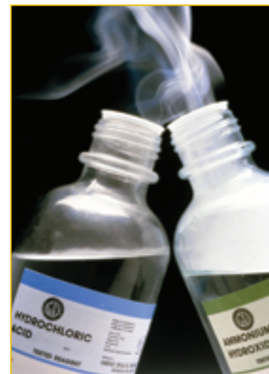
Figure 7.4 Reaction of ammonia gas with hydrogen chloride gas, diffusing from the bottles, to give a white smoke of ammonium chloride. (Note that the name ammonium hydroxide on the bottle is usually written as ammonia solution.)
