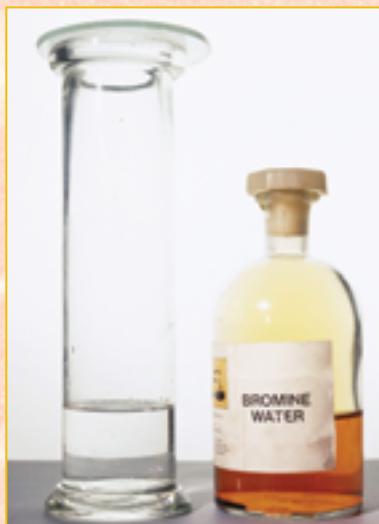
Figure 11.6 Some orange-coloured bromine water was added to ethene (a colourless gas) in a gas jar. Very rapidly, the bromine solution becomes colourless.
