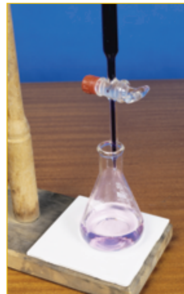
Figure 8.15 Redox titration between potassium permanganate and iron(II) sulfate
