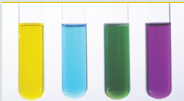
Figure 9.15 The test tubes from left to right contain solutions of VO_2Cl , VOCl_2 , VCl_3 and VSO_4
