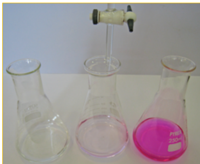
Figure 8.14 During a titration of hydrochloric acid with sodium hydroxide solution, using phenolphthalein as the indicator, the colours shown from left to right are before the end point, at the end point and after the end point.
