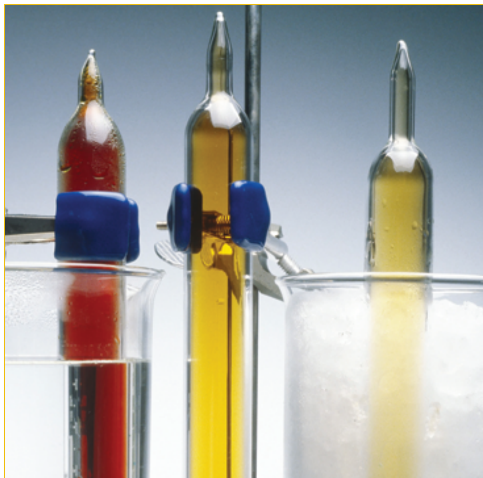
Figure 6.19 The centre sealed tube contains an equilibrium mixture of \text{NO}_2 and \text{N}_2\text{O}_4 . The tube on the left has been heated and the one on the right has been cooled, causing shifts in the equilibrium positions.
