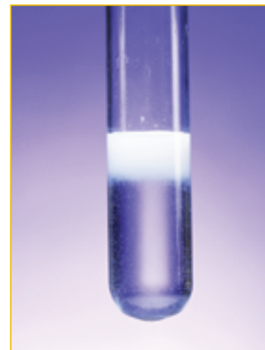
Figure 5.4 A precipitate of silver bromide formed from mixing the two colourless solutions of silver nitrate and sodium bromide
