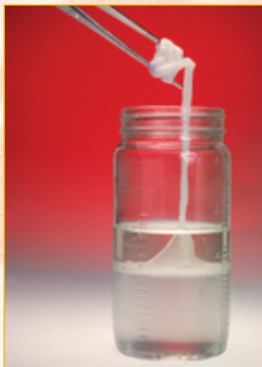
Figure 13.7 Making nylon. The nylon fibre forms at the interface between the two solutions containing the diamine and the dicarboxylic acid.
