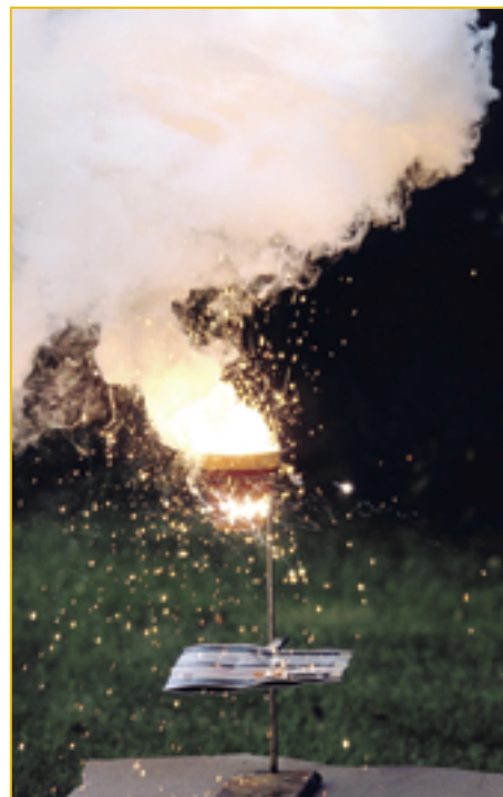
Figure 6.7 The thermite reaction. Sparks of molten iron and a cloud of aluminium oxide can be seen.
