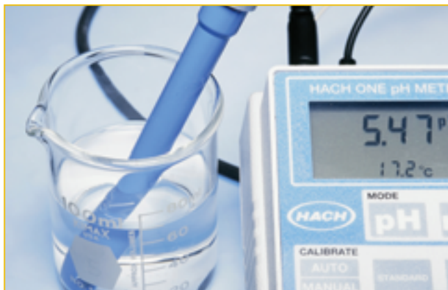
Figure 7.11 A pH meter being used to measure the pH of water containing some dissolved carbon dioxide. Why is the pH lower than 7?
