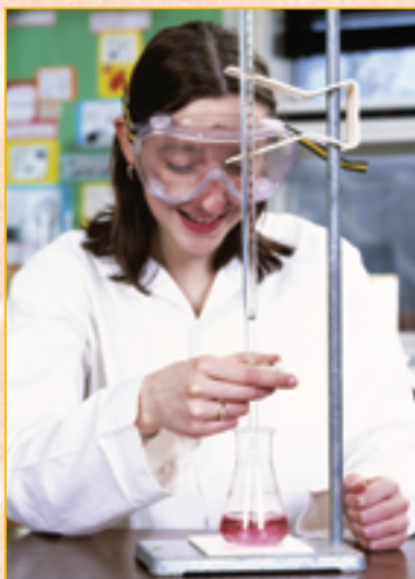
Figure 8.8 Acid being added from a burette to an alkaline solution in the flask. The indicator in this titration is phenolphthalein.
