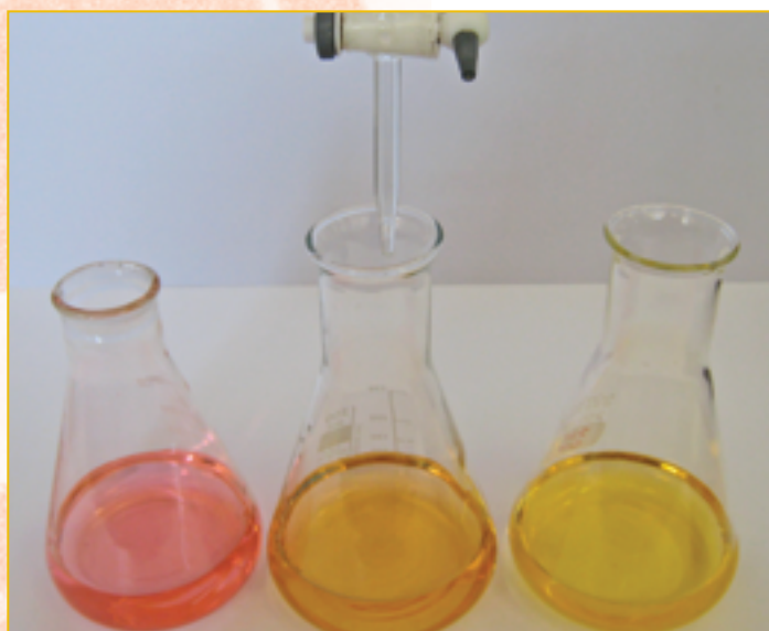
Figure 8.13 During a titration of hydrochloric acid with sodium carbonate solution, using methyl orange as the indicator, the colours shown from left to right are before the end point, at the end point and after the end point.
