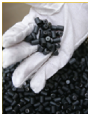
Figure 1.3 Nuclear fuel pellets made from uranium dioxide. The pellets will be loaded into fuel rods and then used in a nuclear reactor to create a controlled nuclear reaction and generate electricity.
