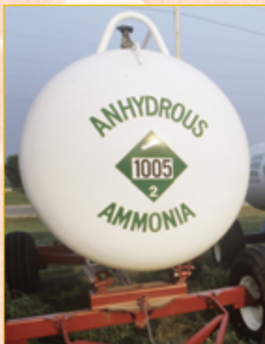
Figure 6.27 Hazard label for stored bulk ammonia
