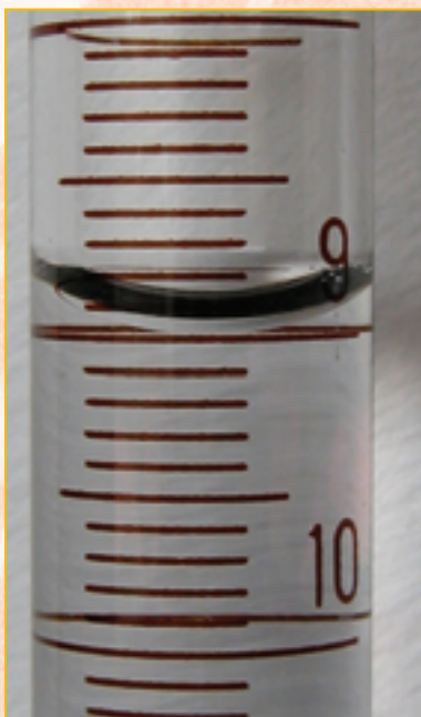
Figure 8.9 For colourless or pale-coloured solutions, the reading on the burette scale is taken from the bottom of the meniscus. On this burette, the reading is 9.00 mL.
