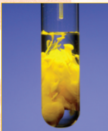
Figure 5.2 A precipitate of lead iodide forms when solutions of lead nitrate and sodium iodide are mixed.
