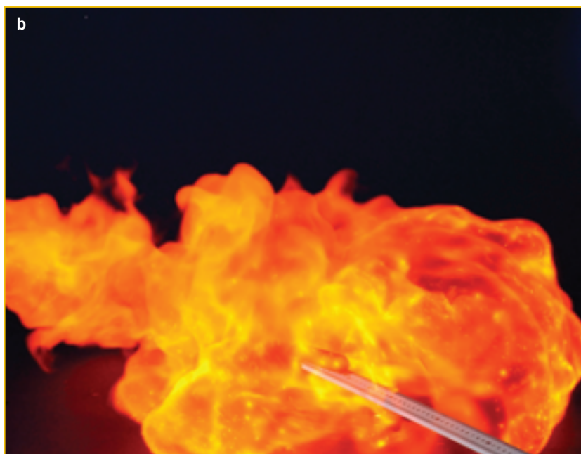
(b) After ignition. The result of igniting the hydrogen/oxygen mixture in the balloon. The explosive reaction between these two gases, once ignited, is very rapid.
